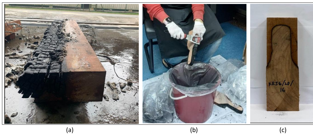
Figure 8 Preparation of charred samples; (a) charred beam before scraping, (b) removing the char on the sliced specimen and (c) comparison between charred cross-section and original cross-section.
