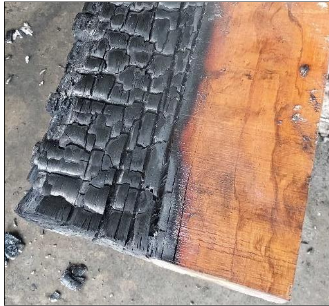
Figure 1 The char layer and unheated timber.
