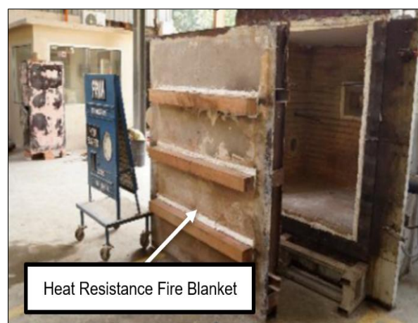
Figure 3 Furnace cover with slotted specimen placement.
