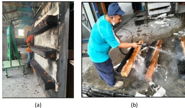
Figure 7 After fire test ;(a) frame was removed from furnace and ; (b) samples were sprayed with water.
