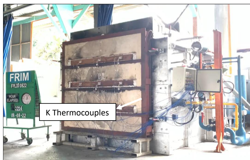
Figure 6 Fire testing furnace with specimen ready for testing.
