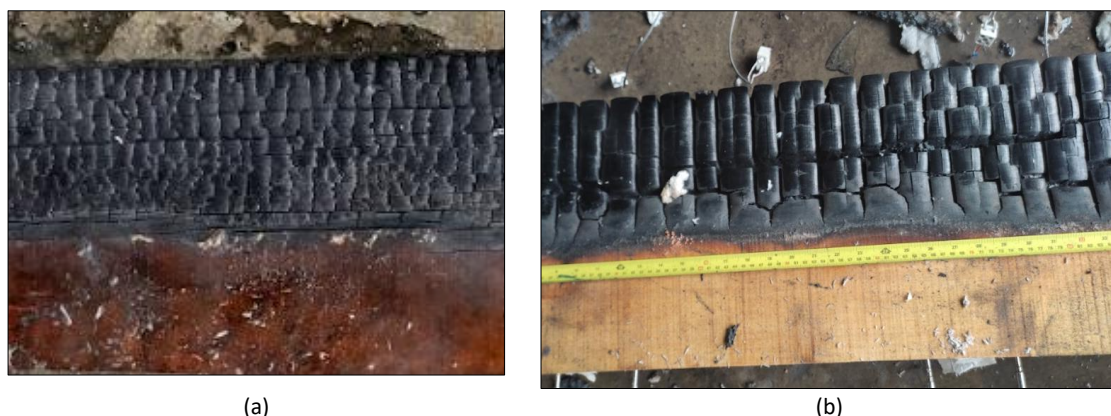
Figure 13 Charring on the lateral surface of; (a) Resak and (b) Jelutong.
