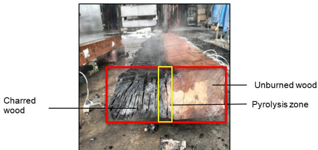
Figure 12 Visual observation after fire test.
