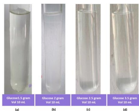
Figure 5 Phase changes of the solution when (a) 1.5 grams, (b) 2 grams, (c) 2.5 grams, and (d) 3.5 grams of glucose were dissolved in a 10 mL mixture of 50%-v water and 50%-v acetonitrile.
