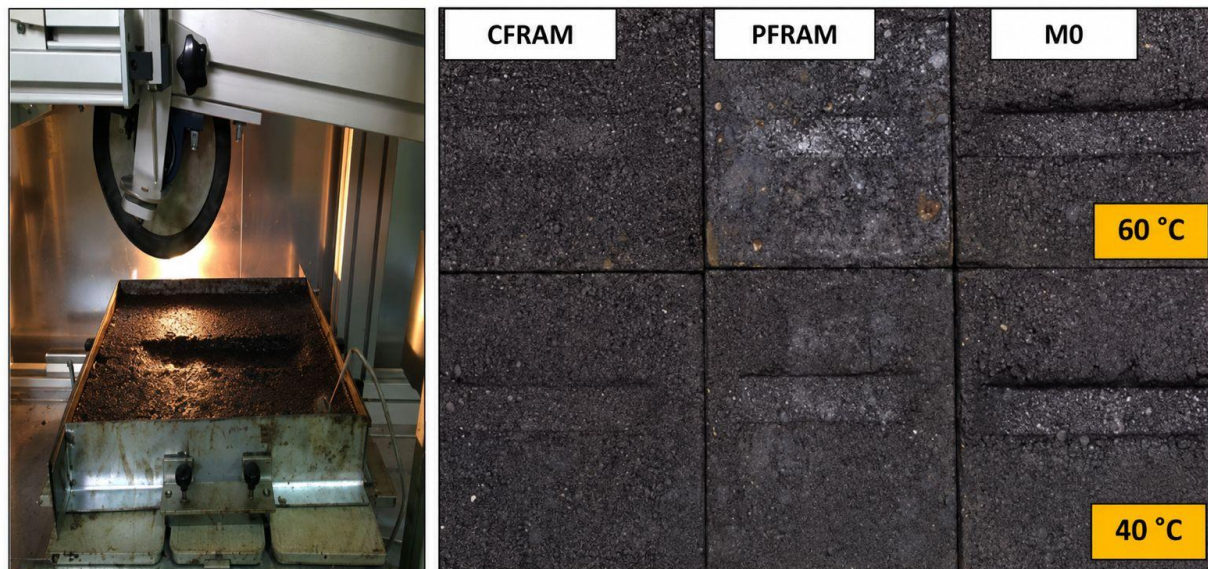
Figure 4 Wheel tracking samples and testing.
