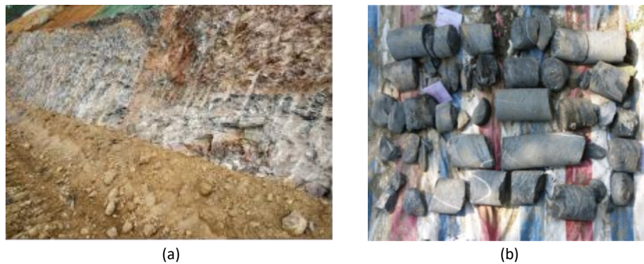
Figure 2 Landslide bed formation site and borehole core: (a) slip bed sandstone, (b) slip bed limestone core.
