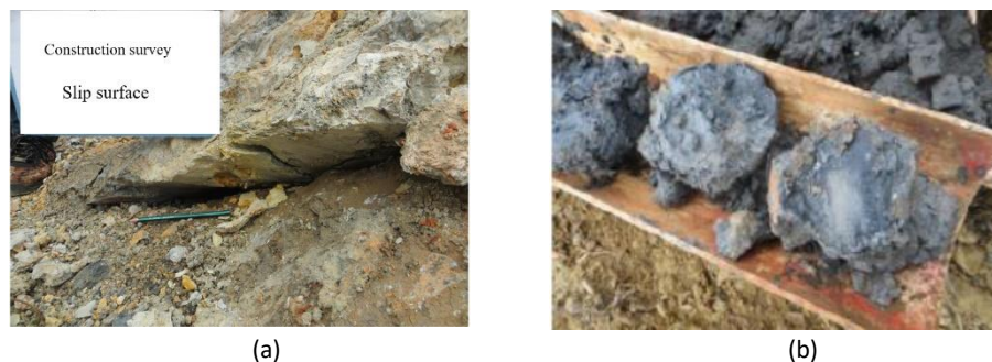
Figure 3 Slip surface and drilling core at shear outlet: (a) cut of the slip surface at the exit, (b) sliding surface drilling shale core.
