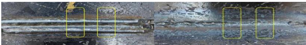
Figure 4 Specimen 3 weld bead and root pass.
