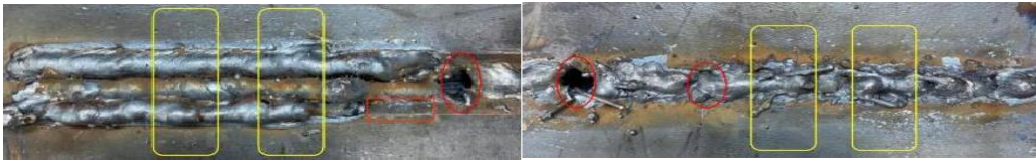
Figure 10 Specimen 9 weld bead and root pass.
