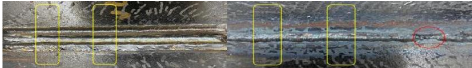
Figure 2 Specimen 1 weld bead and root pass.
