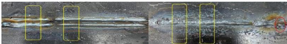
Figure 6 Specimen 5 weld bead and root pass.
