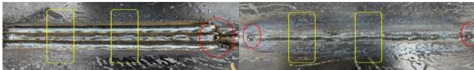
Figure 3 Specimen 2 weld bead and root pass.
