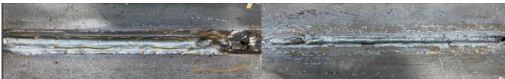
Figure 7 Specimen 6 weld bead and root pass.
