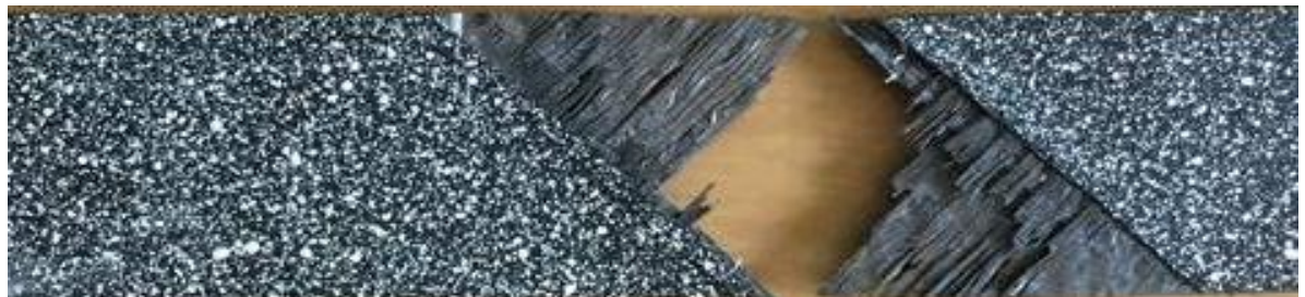
(b) Composite material with orientation (±45°
