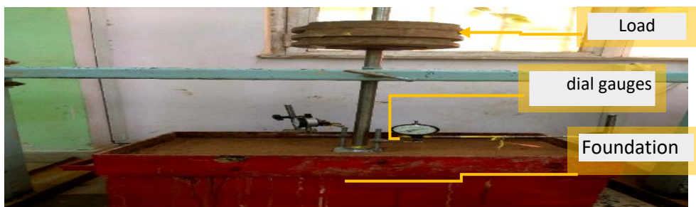
Figure 3 Model test set-up.
