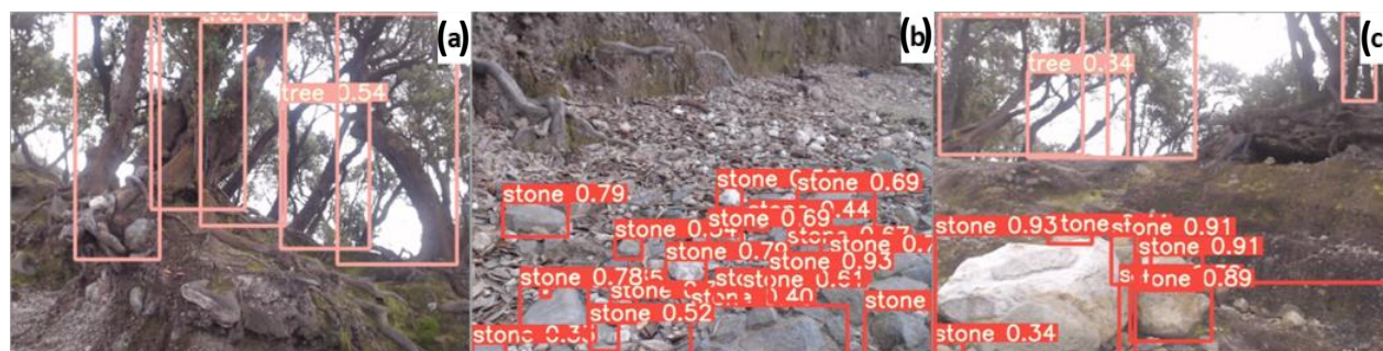
Figure 8 Detection result of Raspberry Pi implementation at Ratu Crater of Tangkuban Parahu Volcano for trees and stones (a), trees (b), and stones (c).
