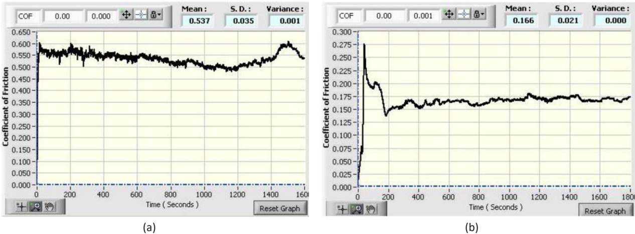
Figure 6 Graph of coefficient of friction (CoF) for (a) stainless steel disc, (b) mild steel disc.
