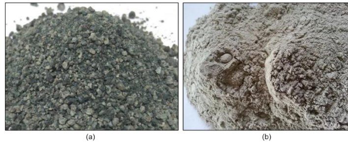
Figure 1 Visual appearance of (a) FS and (b) FA specimens from Obi Island ferronickel plant.
