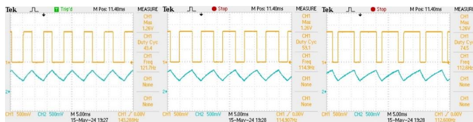
Figure 12 Pulse signal of the IC NE555 for the MOSFET drive at 1,000 rpm, 1,500 rpm, and 2,000 rpm.
