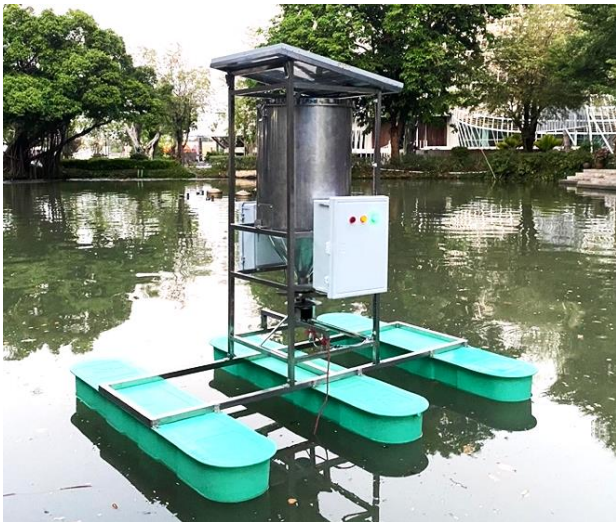
Figure 10 The solar-powered automatic shrimp feeder.
