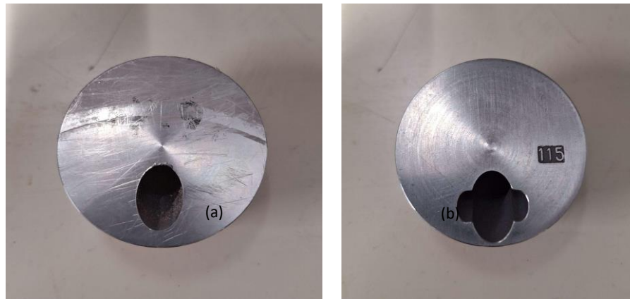
Figure 3 Photographs of nozzle between sub-chamber and main chamber: (a) round shaped nozzle and (b) special shaped nozzle.
