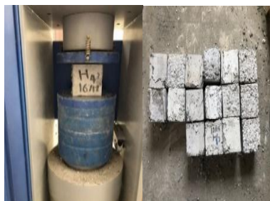
Figure 6 Cube compression test
