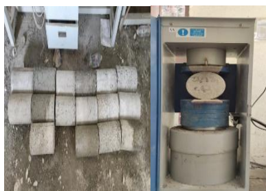
Figure 7 Cylinders splitting tensile test
