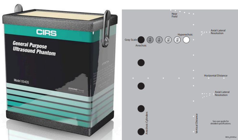
Figure 5 CIRS 054 GS general-purpose ultrasound phantom CIRS 054GS
