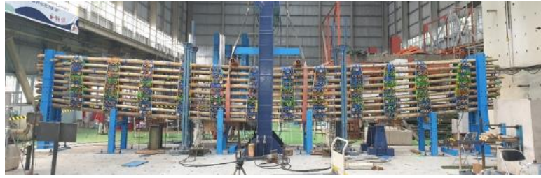
Figure 7 Documentation of bamboo mattress laboratory test.
