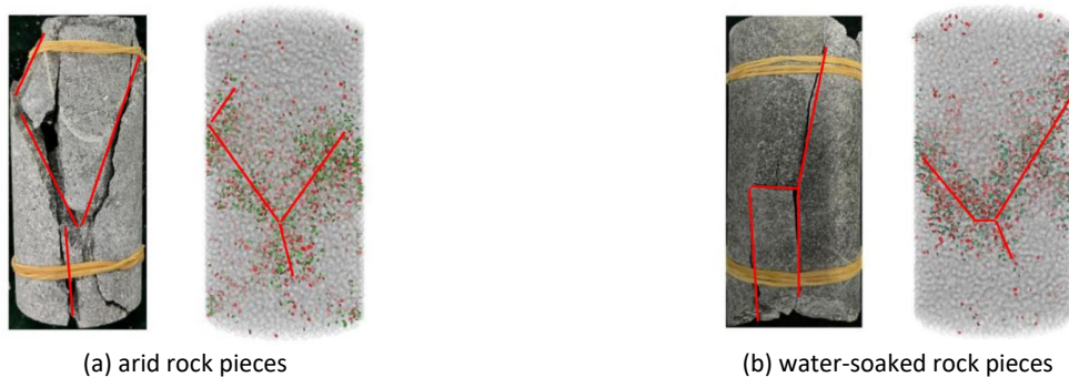
Figure 13 Comparison between experimental and simulated failure patterns of rock pieces.
