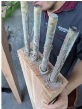
(a) injected epoxy-resin and steel rods embedding
