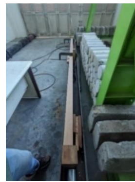
(b) beam clamped using a hydraulic jack
