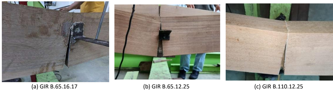
Figure 10 Failure mechanism of timber beam with glued-in rod joints.
