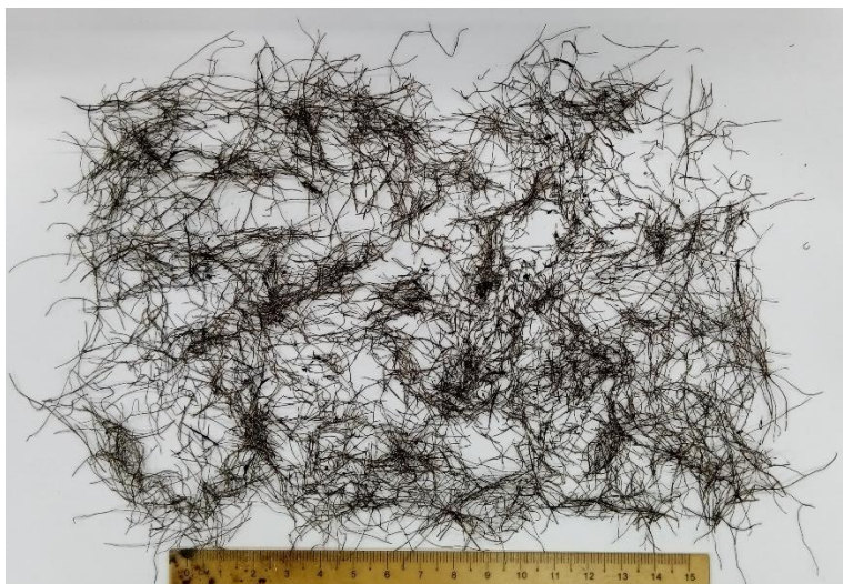
Figure 1 Waste tyre metal fibre used in this research.
