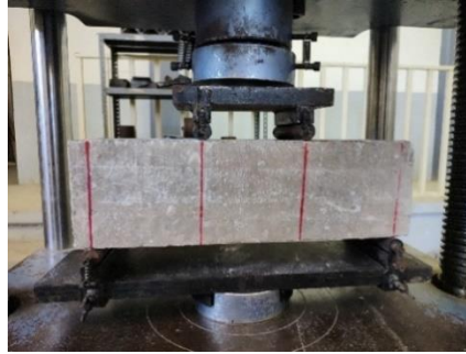
Figure 7 Flexural strength test.
