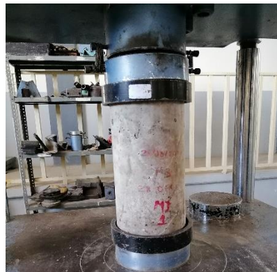
Figure 6 Compressive strength test.
